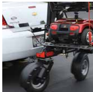
Swivel wheels, independent suspension.
