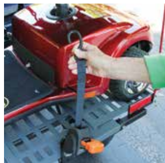
Self-tensioning retractable securement belts.
